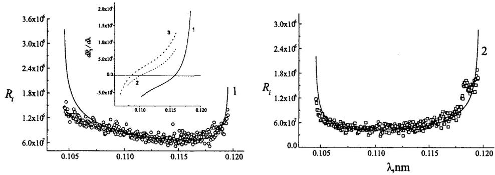
Fig.4. The energetical dependences of a reflectivity for GaAs crystals doped with Si.  $C_{Si}$  are equal 1
