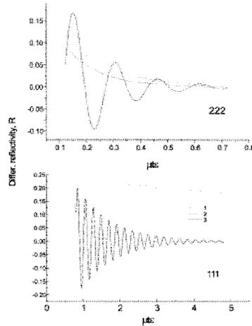
Fig.1. Calculation of the Pendellösung phenomenon for the 222 QFR and “usual” 111 reflection for a GaP perfect crystal (formula 1). Dashed and dotted lines correspond to the Bloch waves with low and strong absorption of X-ray ( $\lambda=1.1984 \text{ \AA}$ )
