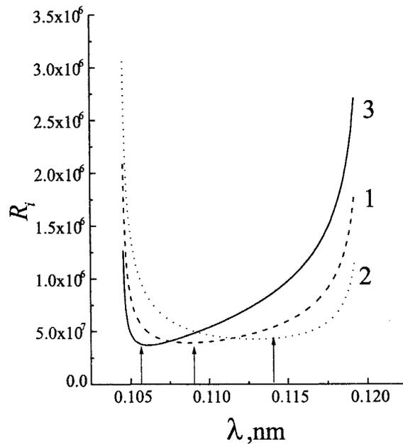
Fig.5. Effect of Ga(2) or As(3) excess on the reflectivity minimum close to the point where  $F_{rh} \rightarrow 0$ . The stoichiometrical sample is shown by curve 1.
