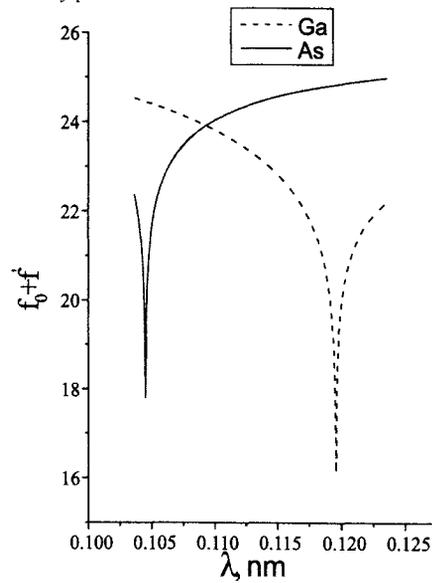
Fig.3. Variations of the Ga and As formfactors with changing of wavelengths between  $\lambda_{\text{KGa}}$  and  $\lambda_{\text{KAs}}$ .
