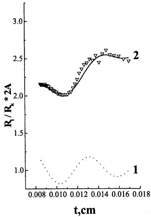
Fig.2. Thickness dependences of a reflectivity for the GaAs crystal containing  $8 \cdot 10^4 \text{ cm}^{-2}$  dislocations (curve 2 ) and for a perfect stoichiometric sample (calculation) (curve 1 ).  $\lambda = 1.1984 \text{ \AA}$ . The experimental results are shown by points.
