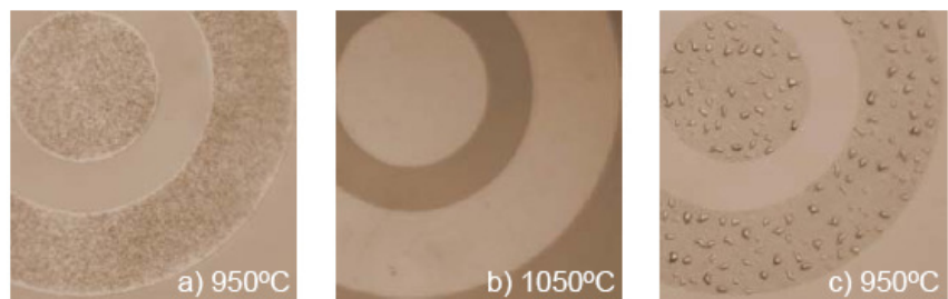
Fig. 4. Optical micrographs of annealed contacts: (a) Ni/n-SiC; (b) \text{Ni}_2\text{Si}/\text{n-SiC} ; (c) \text{NiSi}_2/\text{n-SiC} .
