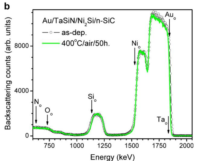
Fig. 3. The 2 MeV He<sup>+</sup> backscattering spectra of the Au/Ni<sub>2</sub>Si/n-SiC (a) and Au/Ta<sub>35</sub>Si<sub>15</sub>N<sub>50</sub>/Ni<sub>2</sub>Si/n-SiC (b) contacts before and after aging in air at 400 °C for 50 h.
