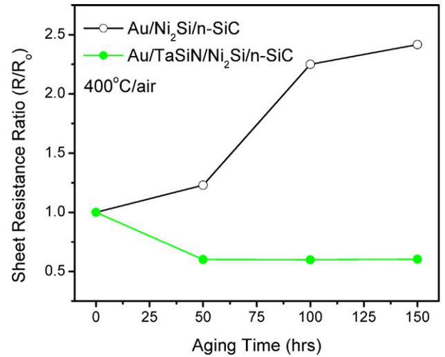
Fig. 2. Thermal stability test for Au/Ni<sub>2</sub>Si/n-SiC and Au/Ta<sub>35</sub>Si<sub>15</sub>N<sub>50</sub>/Ni<sub>2</sub>Si/n-SiC contacts aged in air at 400 °C: variation of contacts sheet resistance (*R/R*<sub>0</sub>) as a function of aging time.
