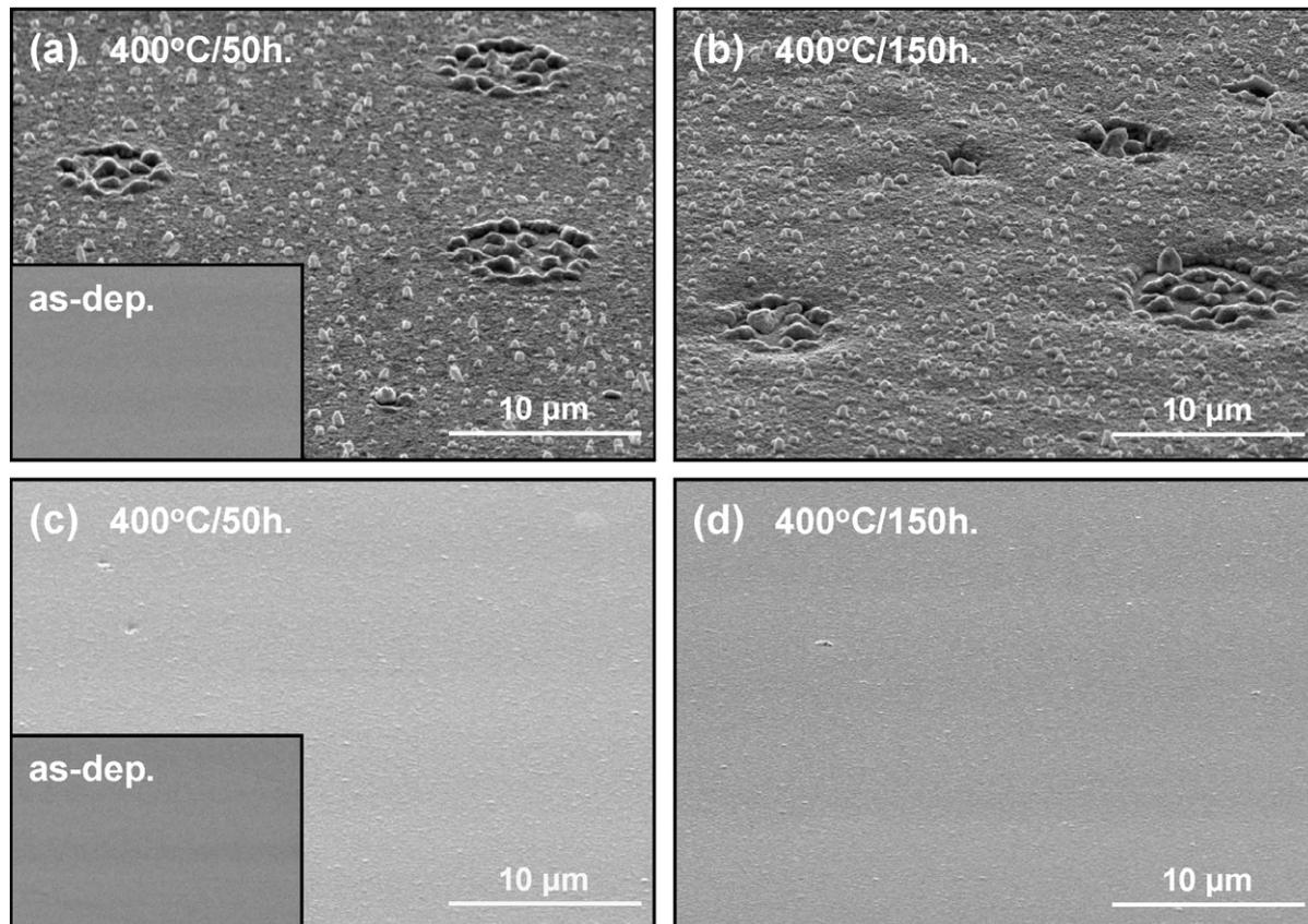
Fig. 4. SEM micrographs of the Au/Ni<sub>2</sub>Si/n-SiC (a and b) and Au/Ta<sub>35</sub>Si<sub>15</sub>N<sub>50</sub>/Ni<sub>2</sub>Si/n-SiC (c and d) contacts: (a, c) as-deposited and after aging in air at 400 °C for 50 h; (b, d) aged in air at 400 °C for 150 h.
