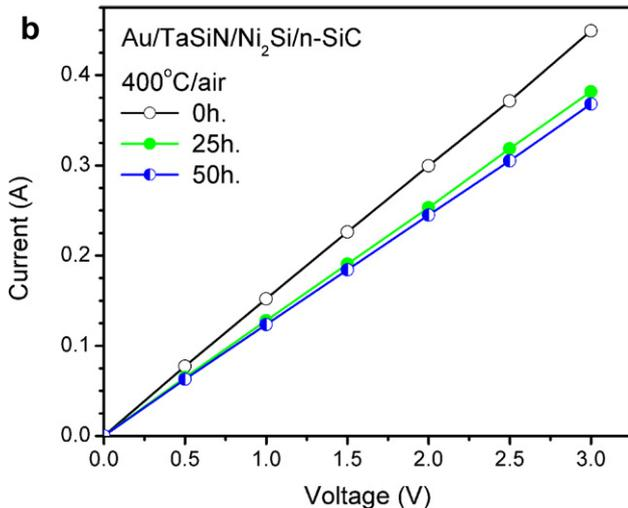
Fig. 1. *I-V* characteristics of the Au/Ni<sub>2</sub>Si/n-SiC (a) and Au/Ta<sub>35</sub>Si<sub>15</sub>N<sub>50</sub>/Ni<sub>2</sub>Si/n-SiC (b) contacts before and after aging in air at 400 °C up to 50 h.
