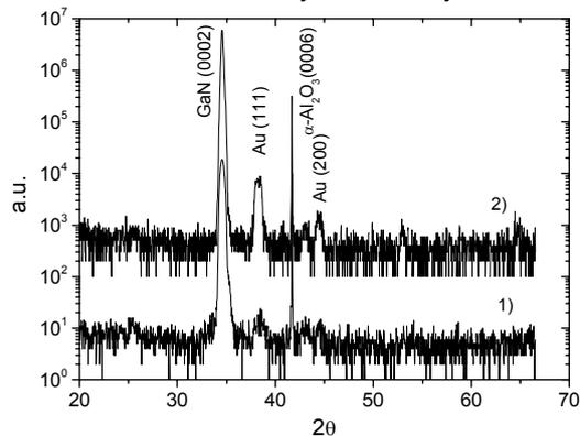
Fig. 3. XRD patterns of the Al<sub>2</sub>O<sub>3</sub>- $n$ -GaN-TiB<sub>x</sub>-Au contact before (1) and after RTA at  $T=870\ ^\circ\text{C}$  for 30 s (2)
