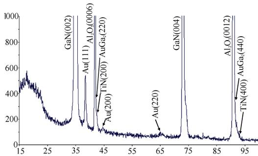
Fig. 2. XRD patterns of the GaN-Ti-Al-TiB<sub>x</sub>-Au contact
