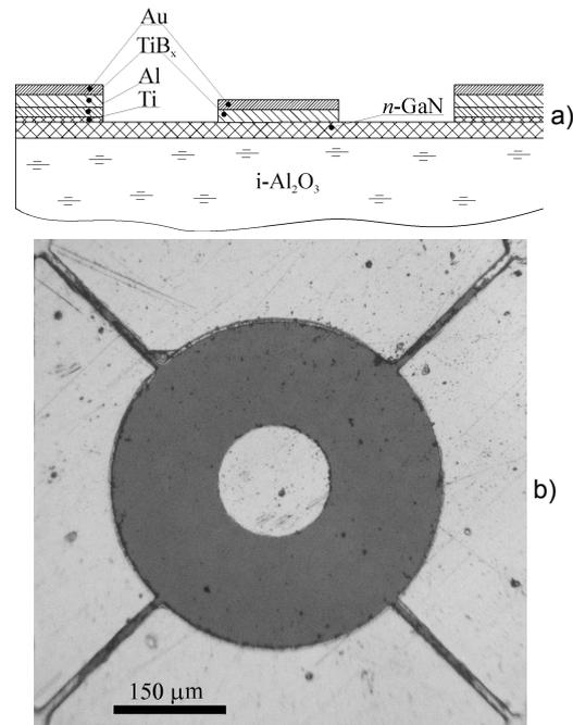
Fig. 1. Layered structure of the contacts (a) and layout of the diode structure (b)
