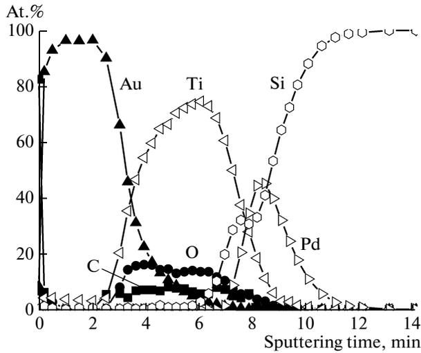
**Fig. 4.** Distribution profiles for components in the ohmic contact Au–Ti–Pd<sub>2</sub>Si–*n*-Si after rapid thermal annealing at  $T = 300^\circ\text{C}$ .
