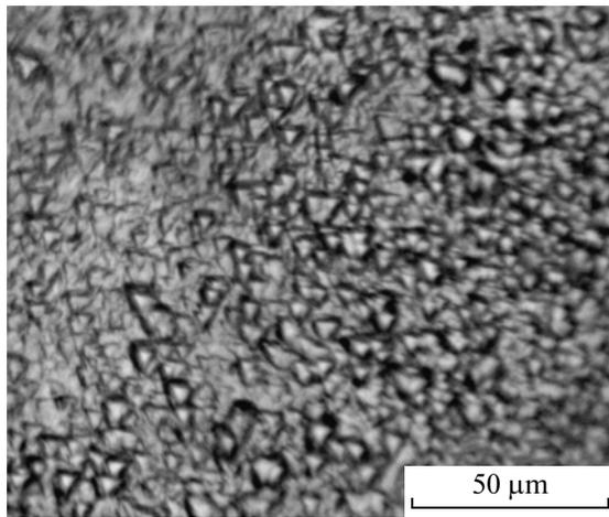
**Fig. 1.** Microstructure of the lapped surface of an *n*-Si wafer after selective etching.
