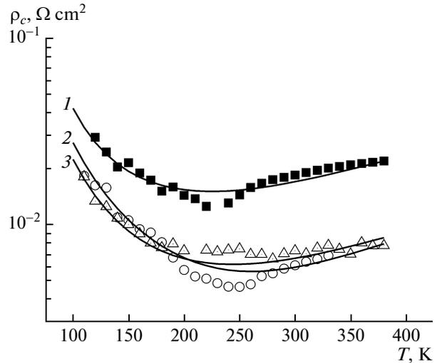
**Fig. 5.** Temperature dependences of  $\rho_c$  for Au–Ti–Pd<sub>2</sub>Si–*n*-Si ohmic contacts: solid lines represent theory and symbols correspond to experimental data for samples 1–3 (curves 1–3, respectively).  $N_d = (1) 5 \times 10^{16}$ , (2)  $3 \times 10^{17}$ , and (3)  $8 \times 10^{17} \text{ cm}^{-3}$ .
