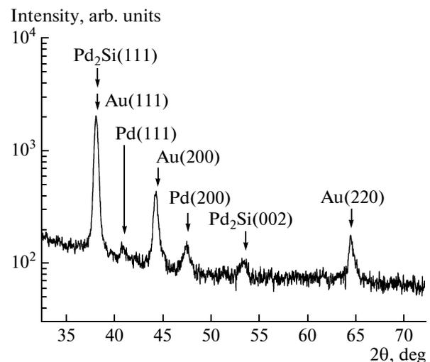
**Fig. 3.** X-ray diffraction patterns of contact metallization Au–Ti– $\text{Pd}_2\text{Si}$ –*n*-Si deposited onto a lapped *n*-Si wafer heated to 300°C.
