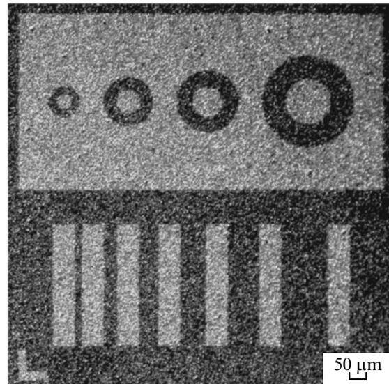
**Fig. 2.** Test structure for measuring the specific contact resistance. Fragment of a TLM structure  $N_{D1} = 7 \times 10^6 \text{ cm}^{-2}$ .
