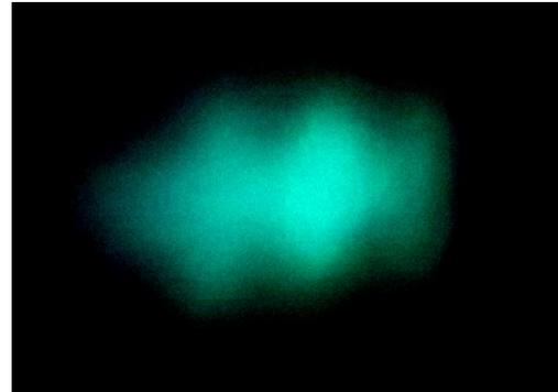
Fig. 1. Imprinted image of a projected to a sample face a razor blade opening. The picture was taken 1 s after switching off the illumination.
