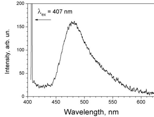
Fig. 4. Polyamide-6 luminescence with the excitation from diode laser at 407 nm.
