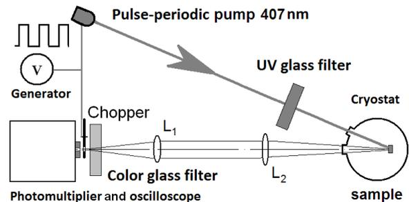
Fig. 5. Experimental scheme composed from the excitation laser diode (407 nm) operating in a pulse-periodic regime, sample in a cryostat and a detector (photomultiplier). The chopper closes the photomultiplier window at the moments of the excitation pulses and opens it in the interval between the pulses.
