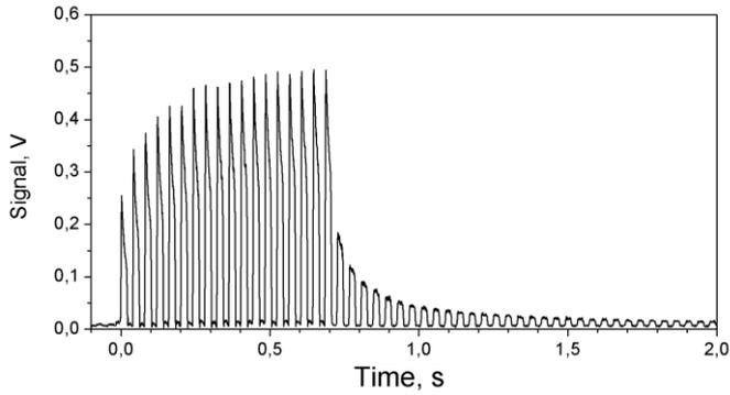
Fig. 6. Example of experimentally recorded time-delayed luminescence signal at room temperature. Excitation from a diode laser (407 nm) lasts to 0.7 s, then the relaxation of the afterglow signal is detected with a hyperbolic function.
