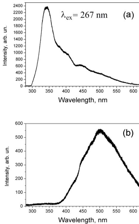
Fig. 3. Comparison of the luminescence spectra of the Polyamide-6 samples in the crystalline form  $\alpha$  (a) and  $\gamma$  (b).
