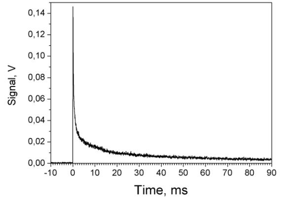
Fig.8. Luminescence response of Polyamide-6 sample ( $\alpha$ -form) on UV pulse pump from  $N_2$  laser (337 nm, 9 ns duration) at room temperature. The sharp peak is a direct response (fluorescence) spike. Long-time afterglow “tail” signal is seen.
