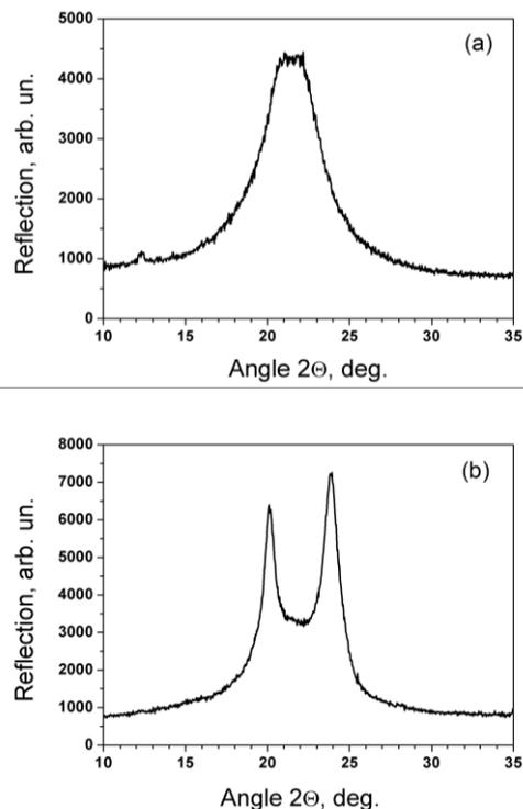
Fig. 2. Wide-angle X-ray diffraction pattern of polyamide-6 samples in  $\gamma$  (a) and  $\alpha$  (b) forms.
