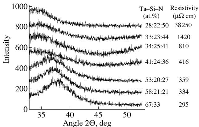
**Fig. 1.** X-ray diffraction spectra taken of the as-deposited Ta-Si-N films with a different nitrogen concentration. On the right, atomic ratio Ta : Si : N and the resistivity of the films are shown.
